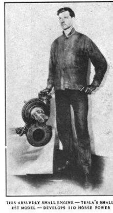
Figure 3: Tesla turbine that used steam as motive agent and developed 110 horse power [4].
